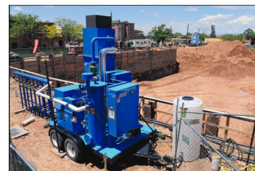
A soil vapor extraction system was used in the clean-up effort at the site for the new Santa Fe County courthouse. Other "brownfields" are scattered around Santa Fe.
